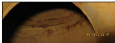
Line 3 at portable pump connection – weld seam contaminated and showing signs of extensive corrosion products
