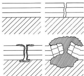
Fig. 1: various stages of rust of mill scales.
